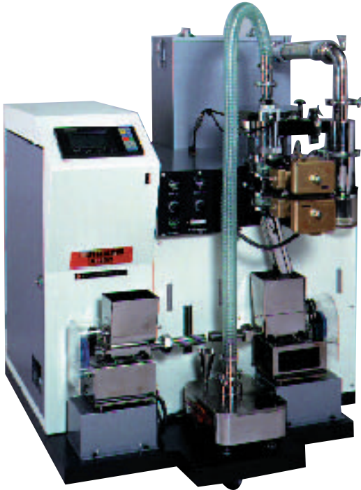
Turbo Classifier TC-15/Current Jet CJ-10 (Laboratory use closed pulverizing and classifying system)
